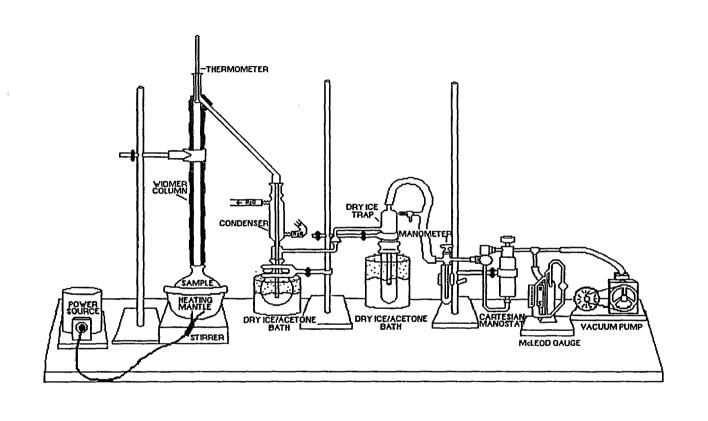
Figure 1. Schematic diagram of FAME distillation apparatus
