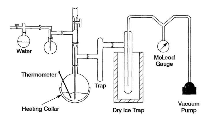
Figure 2. Schematic diagram of oil deodorization apparatus
